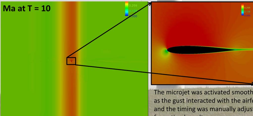
The microjet was activated smoothly as the gust interacted with the airfoil, and the timing was manually adjusted for optimal results.
