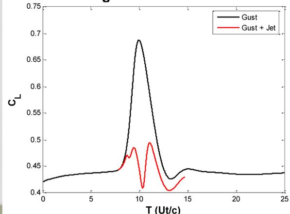
Microjet activation counteracts the effect of a gust convecting with the free stream past a NACA 0012 airfoil.
